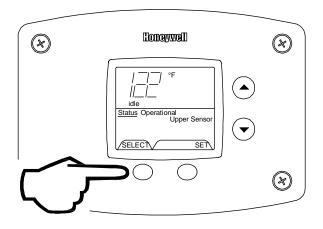
Step 3: For water heaters using two temperature sensors, pressing the "Select" button again displays the Lower Sensor temperature reading. "Lower Sensor" will be displayed in the lower left side of the status window of the water heater display.
